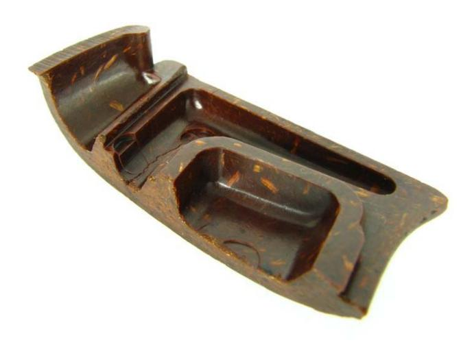
**Conclusion:** It seems that Bakelite is indeed highly resistant to various oils. As was observed after one year, after three plus years there still does not seem to be any breakdown of the Bakelite. Color and texture were indistinguishable from the control piece. Also as noted in year one, the Bakelite is no softer (as tested with a scribe) than the control piece.
